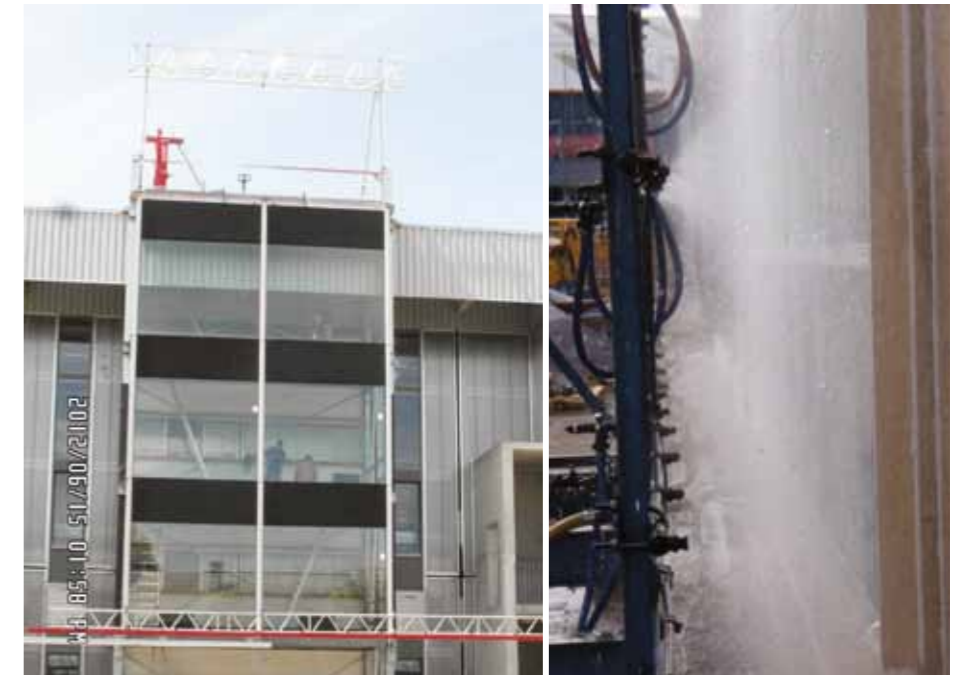
Official test done by IFT Rosenheim, at Lindner's test rig in Arnstorf
